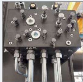
Hydraulic manifold in a manufactured monoblock and cartridge valves
